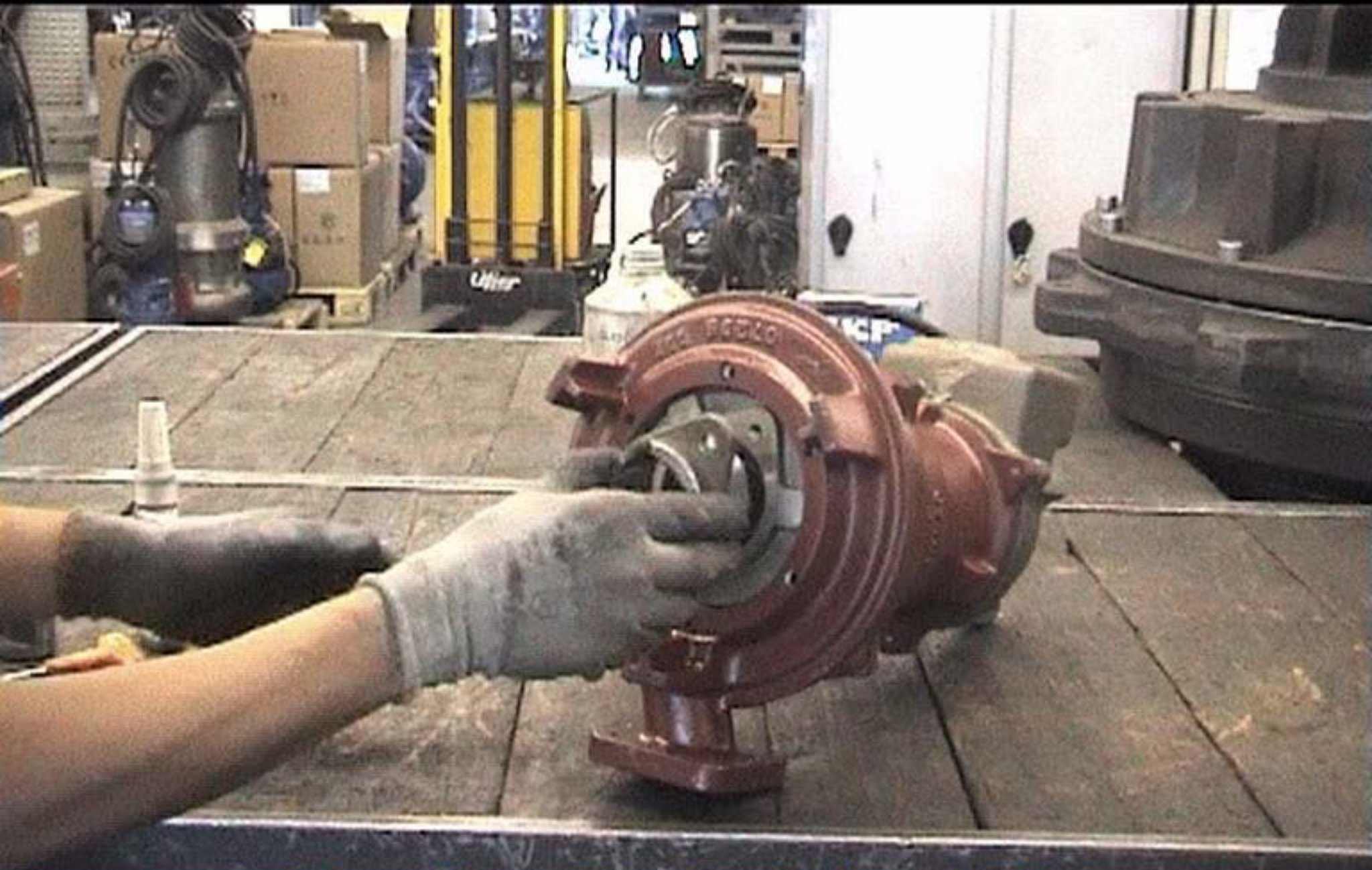
Assemblaggio parte statica grinder Assembly of the static side of the grinder
